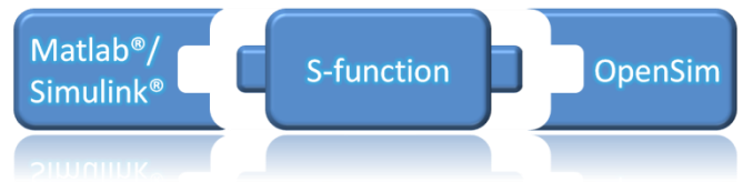
Figure 1: New S-function (system function) interface linking rapid design and control tools of MATLAB®/Simulink® with neuromusculoskeletal dynamic simulation tools of OpenSim.
