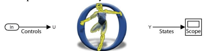
Figure 2: Generic open-loop Simulink® model using the OpenSim-based S-function interface to generate output states (e.g., kinematics) from input controls (e.g., muscle excitations or joint torques).
