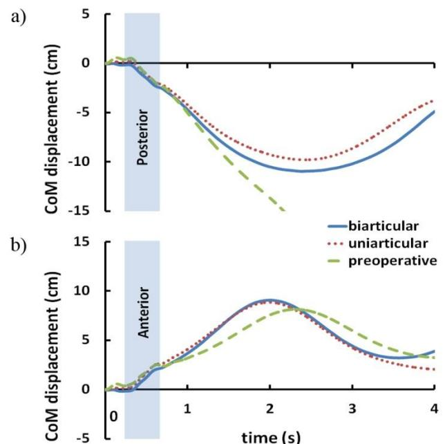
**Figure 3:** Center of mass (CoM) displacements relative to the support-surface translating (a) posterior and (b) anterior for simulations of preoperative, unilateral, and bilateral tendon transfer. The shaded regions highlight the duration of support-surface translations.
