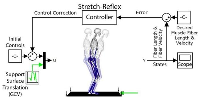
**Figure 2:** Closed-loop Simulink model of balance recovery using a muscle stretch-reflex controller. The controller uses the muscle's fiber length and velocity to generate a control correction to maintain the CoM position above the base of support.
