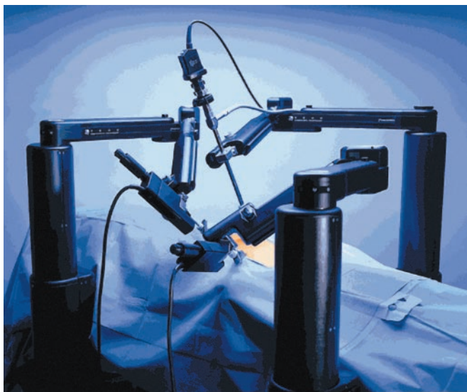
Figure 1. Digital image of the ZEUS Robotic Surgical System arms attached to the standard operating room table rails and positioned around the patient.
