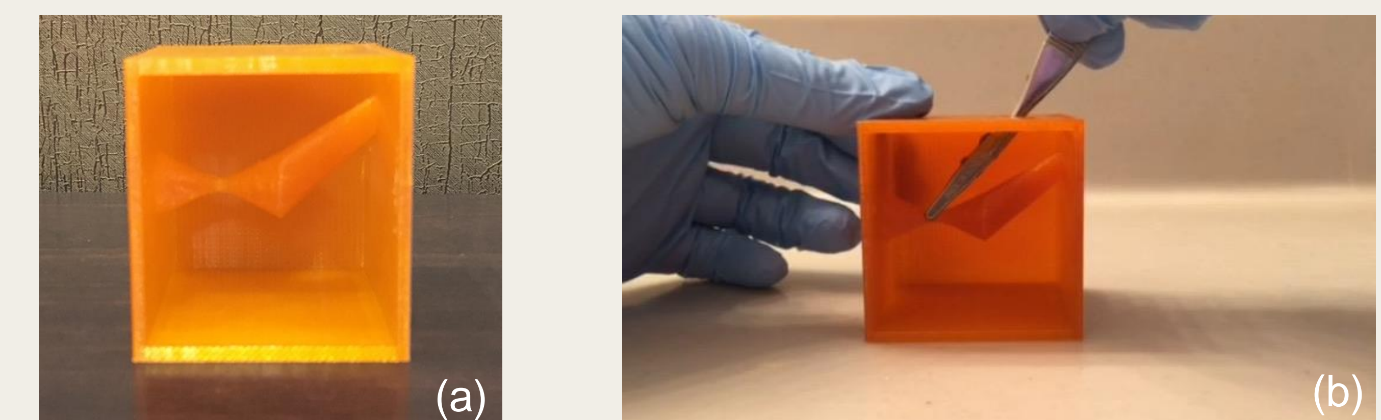
Fig 6: (a) Initial working prototype and (2) the prototype being tested by going through the clipping process
