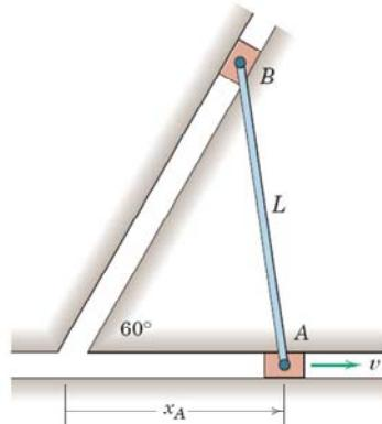
Slider **A** moves horizontally with a constant speed **v**.
