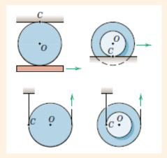
(2) Clearly, when θ = 0, the point of contact has zero velocity so that  $\dot{x} =$  $\dot{y} = 0$ . The acceleration of the contact point on the wheel will also be obtained by the principles of relative motion in Art. 5/6.
