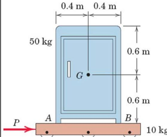
Determine the value of the **force**  $P$  which would cause the cabinet to begin to tip.
