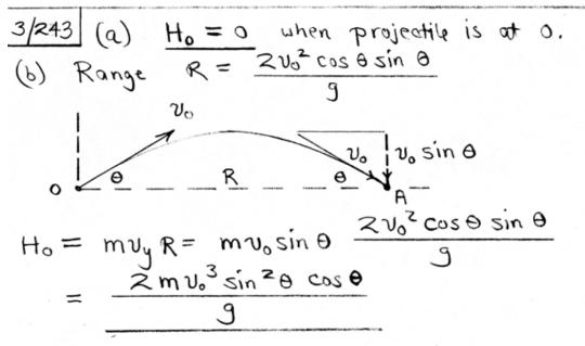
The moment of the projectile weight about point 0 is always increasing the angular momentum ploaut 0.
