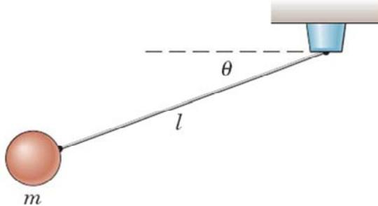
Using only the angular impulse-momentum principle, determine the expression for  $\ddot{\theta}$  in terms of  $\theta$  and the **velocity**  $v$  of the pendulum at  $\theta = 90^\circ$ .
