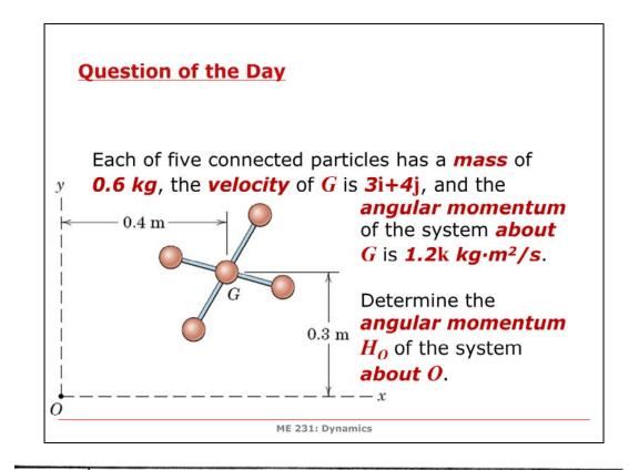
4/12  $H_0 = H_G + \overline{r} \times G$ ,  $G = 3(3\underline{i} + 4\underline{j})$  kg·m/s =  $1.20k + (0.4i + 0.3i) \times 3(3i + 4i)$ = 1.20 k + 3 (1.6 k - 0.9 k) = 1.20 k + 3 (0.7k) = 3.3 k kg·m²/s
