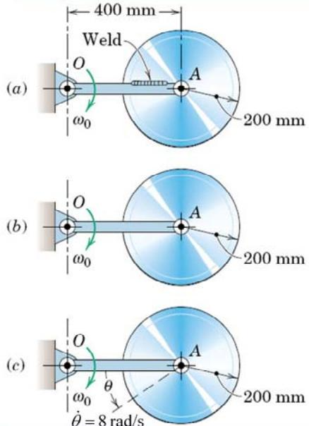
A uniform circular disk has a **mass** of **25 kg** and is mounted to a rotating bar in three different ways and  $\omega_0 = 4 \text{ rad/s}$
