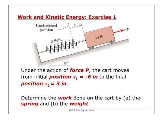
$$\frac{3/104}{(a)} \quad U_{1-2} = \pm k (x_1^2 - x_2^2) \\ = \pm (3)(12) \left[ \left(\frac{6}{12}\right)^2 - \left(\frac{3}{12}\right)^2 \right] = \frac{3.38 \text{ ft-1b}}{3.38 \text{ ft-1b}} \\ (b) \quad U_{1-2} = - \text{mgh} = -14 (\frac{9}{12}) \sin 15^\circ \\ = -2.72 \text{ ft-1b} \end{cases}$$
