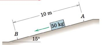
A **50-kg** crate is given an initial **velocity** of **4 m/s** down the chute at **A**. The **coefficient of kinetic friction** is **0.30**.
