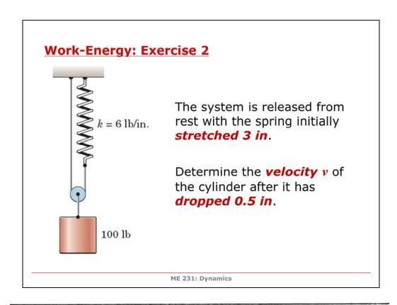
3/154 For the system,  $T_1 + V_1 + U_{1\cdot 2} = T_2 + V_2$   $\pm m_1 v_1^2 + \pm k_1 v_2^2 + o = \pm m_1 v_2^2 + \pm k_1 v_2^2 - mgh$ ,
