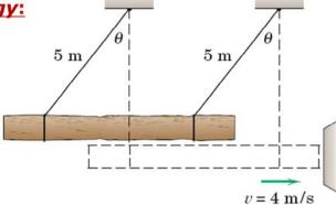
The log is suspended by two parallel 5-m cables and used as a battering ram.
