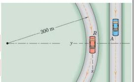
Car A has a **speed**  $v_A$ = 100 km/h, which is increasing at the rate of 8 km/h each second. Car B has a **speed**  $v_B$ = 100 km/h, around the turn and is slowing down at the rate of 8 km/h each second.
