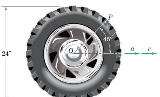
Determine the *velocity* of the truck when point *P* in the *position* shown will have *zero*horizontal component of acceleration.
