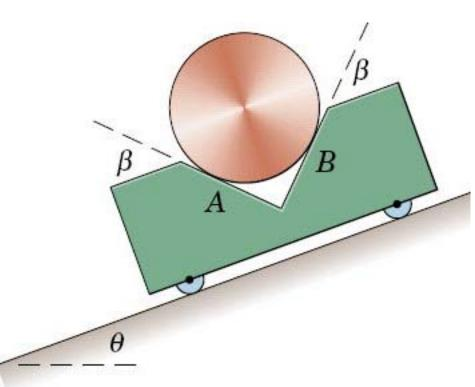
A cylinder rests in a supporting carriage where  $\beta = 45^{\circ}$  and  $\theta = 30^{\circ}$ .
