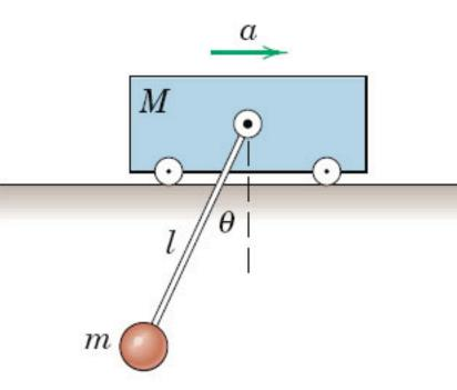
What is the resulting steady-state **angle**  $\theta$  which the freely pivoting bar makes with the vertical?
