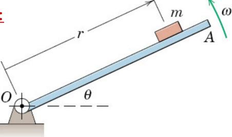
Link OA rotates about a horizontal axis through O with constant angular velocity w = 3 rad/s. When  $\theta = O^{\circ}$ , a small block of mass m is placed on it at a radial distance r = 18 in. When  $\theta = 50^{\circ}$ , the block begins to slip.
