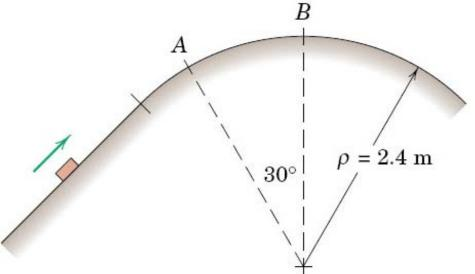
Determine the maximum speed v which the block can have at A without losing contact with the path.
