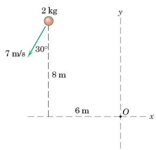
Determine the magnitude  $H_0$  of the **angular momentum** of the **2-kg** sphere about **point 0**.
