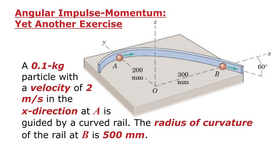
Determine the *time rate of change* of the angular momentum  $H_0$  about the *z-axis* through O at both A and B.
