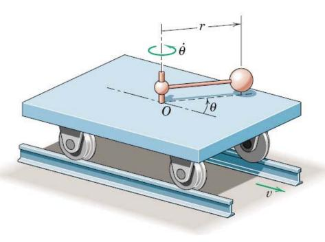
A small *car* with mass of **20** kg rolls freely and carries a **5-kg sphere** mounted on a light rotating *rod* with r = 0.4 m and *angular* velocity of **4** rad/s. The car has a velocity v = 0.6 m/s when  $\theta = 0^{\circ}$ .
