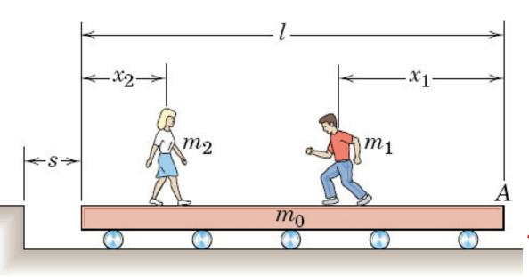
Determine an expression for the **displacement** s of the platform when the two meet **in terms** of  $x_1$  relative to the platform.
