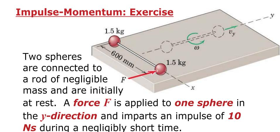
Determine the **velocity** of each sphere as they pass the **dashed position**.
