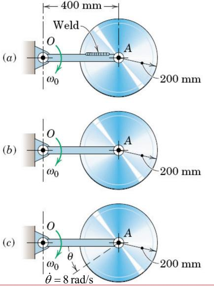
A uniform circular disk has a **mass** of **25 kg** and is mounted to a rotating bar in three different ways and  $\omega_0$ = **4 rad/s**
