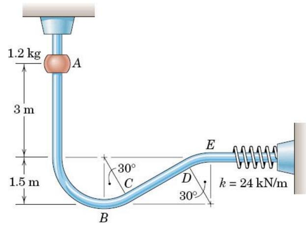
The **1.2-kg** slider is released from rest at **A** and slides without friction along the guide.
