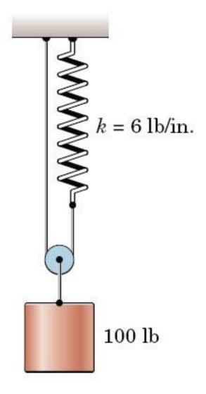
The system is released from rest with the spring initially **stretched 3 in**.
